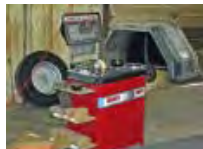
(Left) All the Hart trailer tires are radials and spun balanced.
